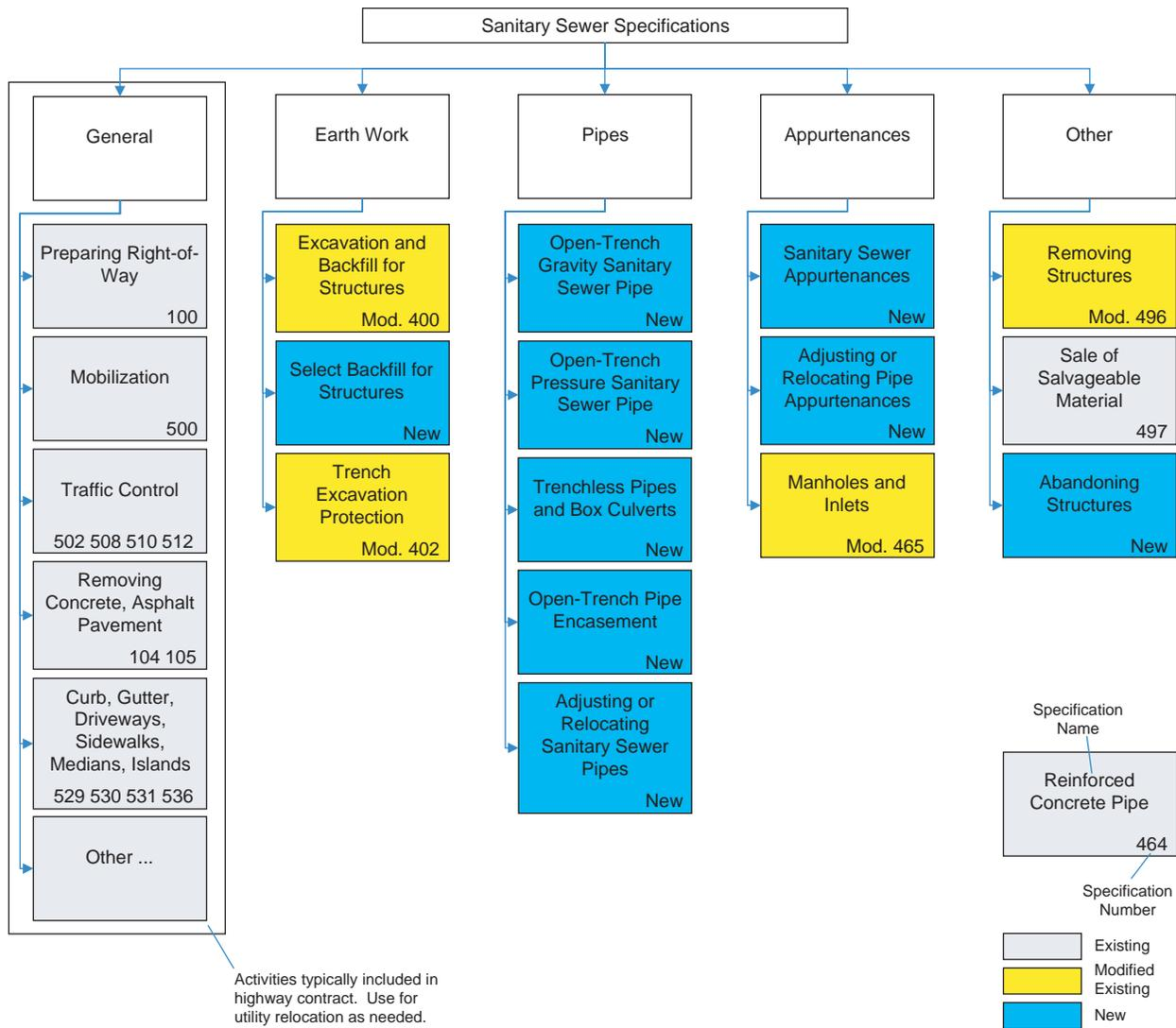
FIGURE 4 Prototype sanitary sewer specification framework.
