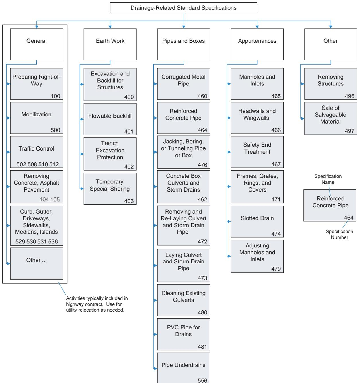
FIGURE 1 Existing drainage-related standard specifications. PVC = polyvinyl chloride. Adapted from TxDOT (9).
