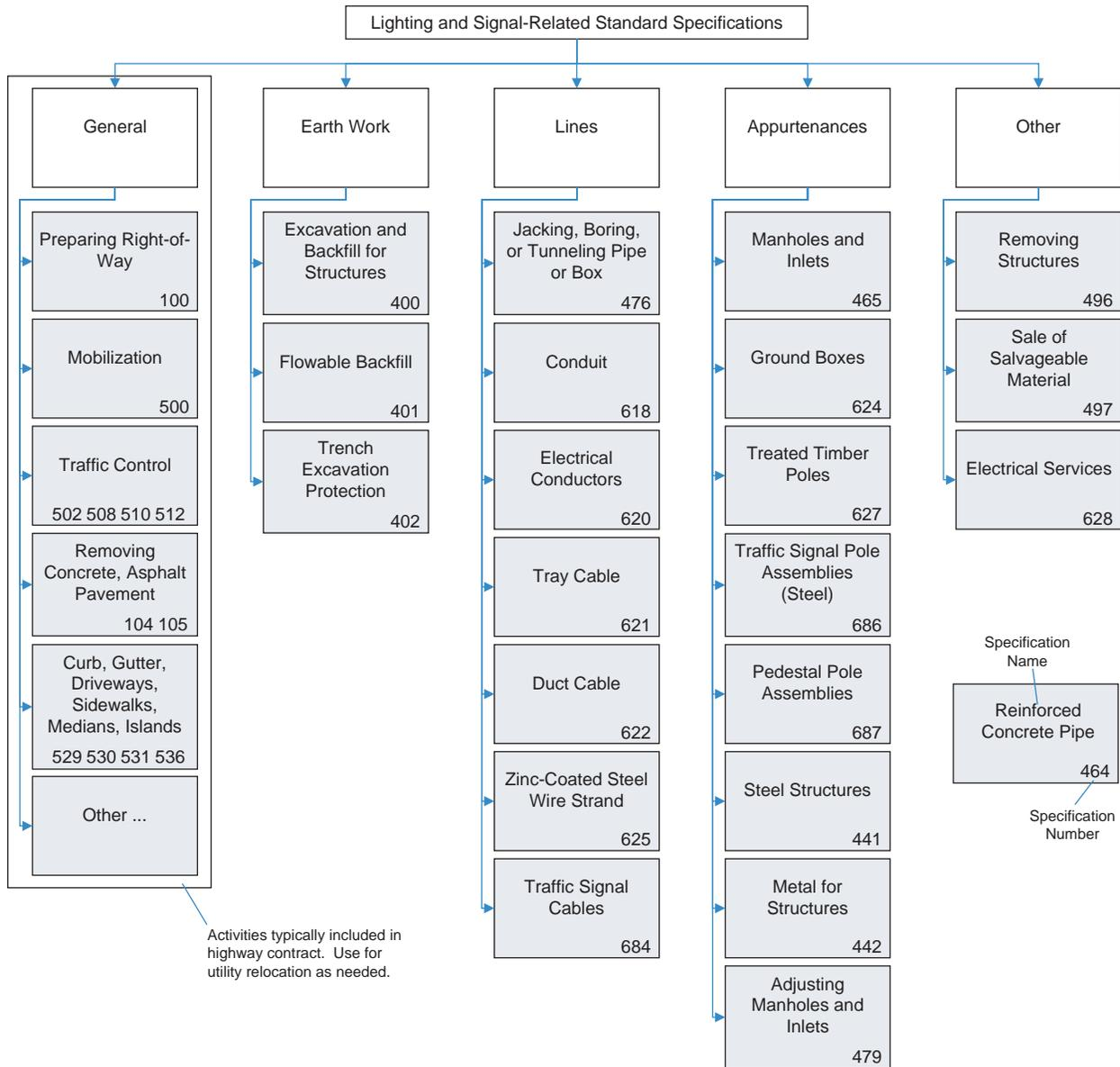
FIGURE 2 Existing lighting and signal-related standard specifications. Adapted from TxDOT (9).
