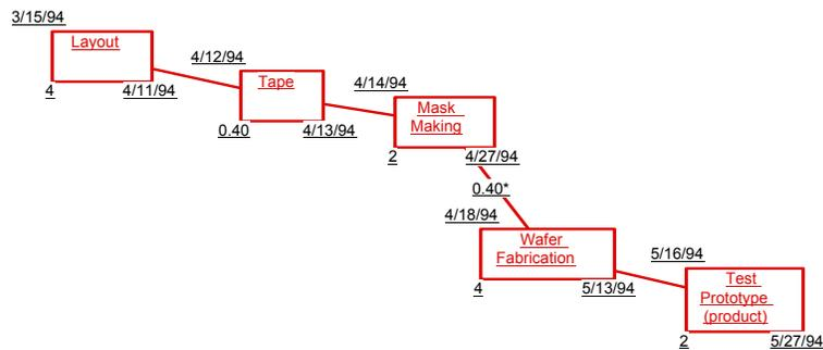
**Figure 5-8: Critical Path Method Estimate of Static Delay between Design and Prototype Test Phases: Activity Chart**
